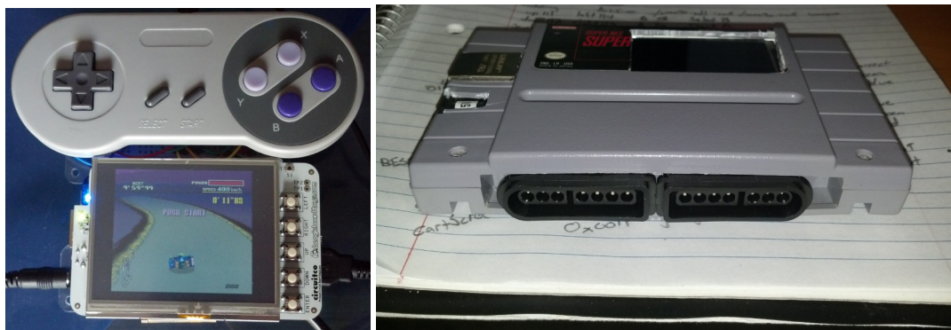
Figure 5.1: Prototypes for a portable BES system (left) and a console unit (right). The portable prototype still requires a USB gamepad and power via the +5VDC barrel connector, so it isn't fully "portable". The console prototype supports native SNES controllers and has a TFT LCD status display.
